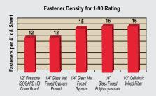
Excellent wind uplift performance means Firestone ISOGARD HD Cover Board requires fewer fasteners than other comparable cover boards.
