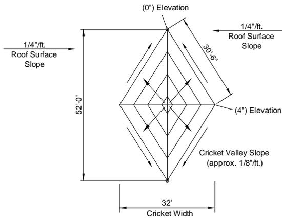
$$\frac{4" \text{ Elevation Difference (} 1/4"/\text{ft. Roof Surface Slope)} \times 16' \text{ (32' cricket width} \times 0.5)}{}$$
