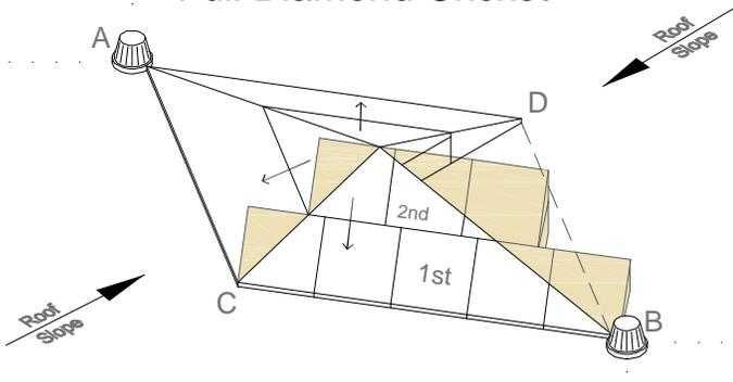
1. Measure the distance between the drains and verify with those on shop drawing.
