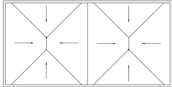
Modified 4 Directional Slope w/drains out of line
