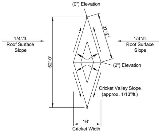
$$\frac{2" \text{ Elevation Difference (} 1/4"/\text{ft. Roof Surface Slope)} \times 8' \text{ (16' cricket width} \times 0.5)}{}$$
