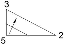
Elevation Difference (roof surface slope x cricket width, points 3 to 5) ÷ Length of Cricket Valley (points 2 to 3)
