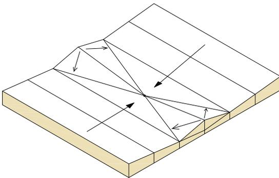
2 Directional Slope to internal Roof drain w/ Crickets
