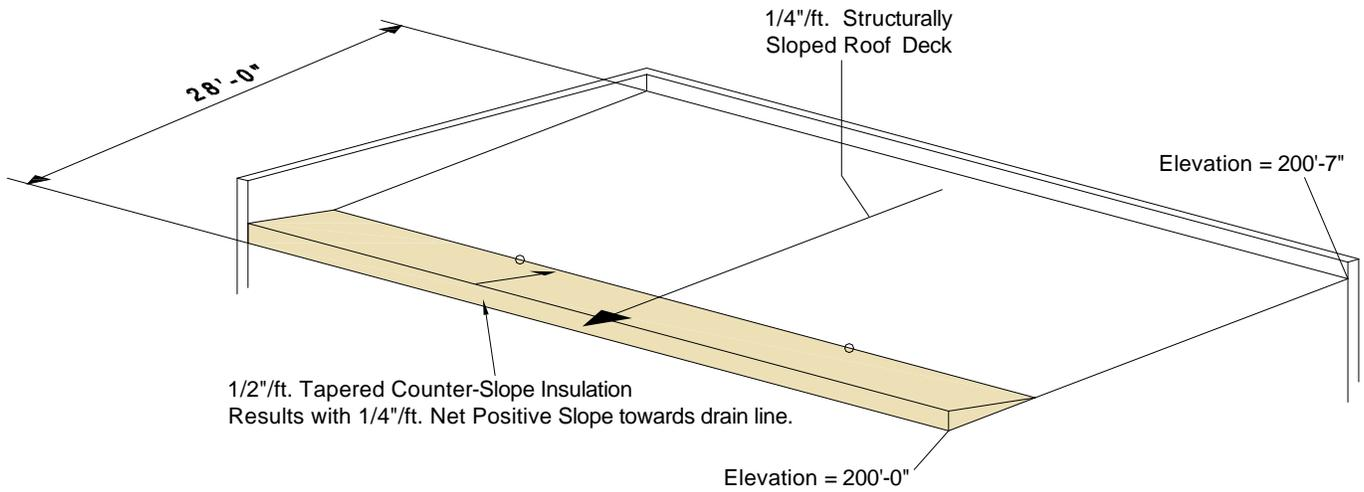
Tapered Counter-Slope Insulation without Crickets
