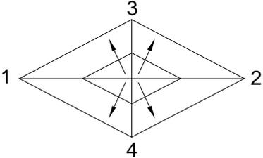
Elevation Difference (roof surface slope x half cricket width, points 3 to 4) ÷ Length of Cricket Valley (points 1 to 3)
