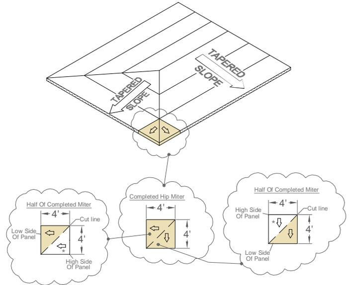
\* The remaining portions left over from the valley miter can be used to create a hip miter, if one is required elsewhere in the tapered layout.
