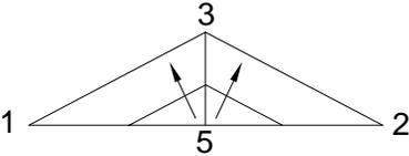
Elevation Difference (roof surface slope x cricket width, points 3 to 5) ÷ Length of Cricket Valley (points 1 to 3)
